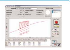
**Oscillation** measures the dynamic viscoelastic properties as a function of frequency. Measurements include single frequency, frequency sweep, amplitude sweep, time sweep and temperature sweep (gradient, step change or profile). Tests can be performed at constant stress or constant strain amplitude (under direct control). Oscillation measurements can be superimposed on steady shear. Partial wave sampling is available.
