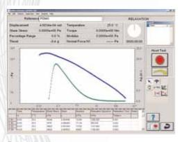
**Relaxation** measures relaxation modulus as a function of time following a step change in strain. The relaxation spectrum and zero shear viscosity can be determined.
