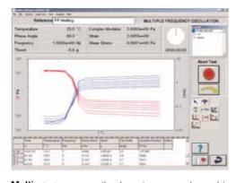
**Multiwave** measures the dynamic response by applying multiple oscillatory frequencies for faster testing. Especially useful for studying rapidly changing systems such as thermosetting resins and for gel point determination.
