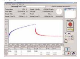
**Creep and Creep Recovery** measures the creep compliance and recoverable compliance as a function of time. User defined sampling modes can be set. Zero shear viscosity and yield stress can be determined.
