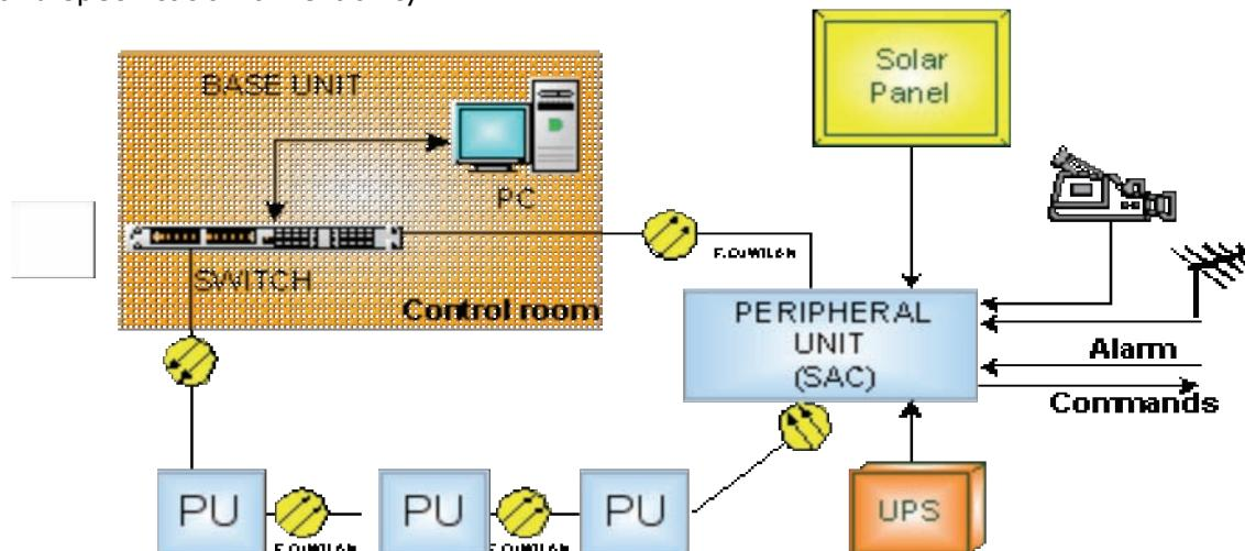
The central element in the PU is the Smart Controller **SAC**.
