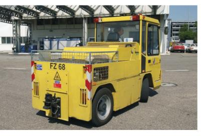
The Rofan BatteryBooster is an electric transport vehicle with nearly unlimited range. This drive system particularly comes into its own where long distances have to be covered also in indoor use (low speeds, low power consumption).
