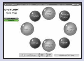
G-Storm's "Home Page" is central to the control of the cycler's various functions. Select the various options, including Program Wizard, New Program, Run Program, on the touch-screen and let the software take you through a logical process that enables you to do what you want to do in easy, simple to follow steps.
