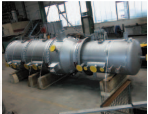
3-stages overhead condenser
