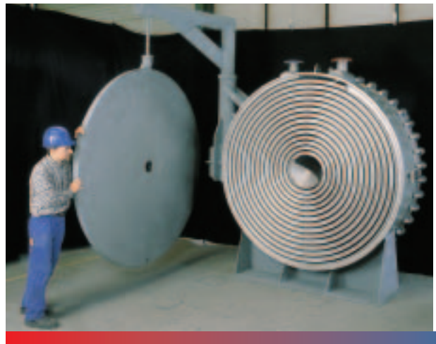
40 m 2 , Ø 1900 mm, Sludge Application
