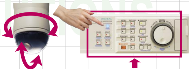
Camera control (PTZ & zoom only) available from the front panel
