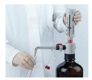
facturing technology to the development and production of bottle-top dispensers. Pistons and cylinders are accurately machined and hand matched to provide a low-wear seal, optimum sliding properties and virtually effortless, onehanded dispensing.
