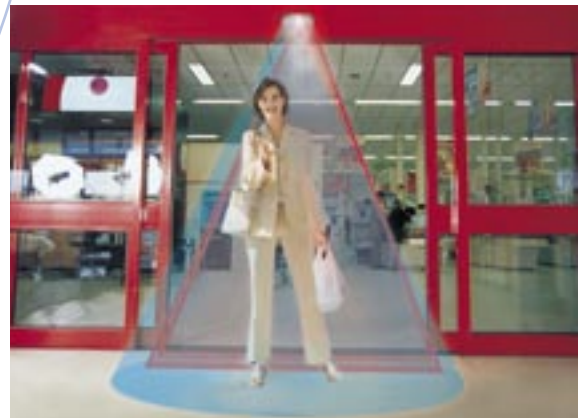
Radar sensing fields (tilt angle 27° with wide field antenna) Safety curtain (tilt angle -4° with narrow field front cover) Mouting height: 2.20 m - 3 elements-antenna
