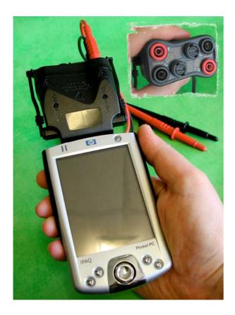
The *Graphic-DMM* is a new concept in test equipment that allows a PDA, Notebook, Tablet-PC and all other Systems equiped with a CF or PCMCIA slot to be turned into a dual channel *Graphic Digital Multimeter* with sophisticated analysis capabilities.
