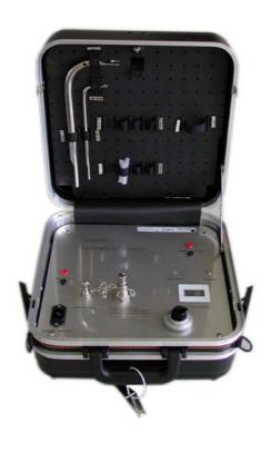
Novasina's newest product, the *CALIBOX*, a mobile calibrator, which allows to generate a very precise and stable pressure in low pressure ranges up to 100 Pa.
