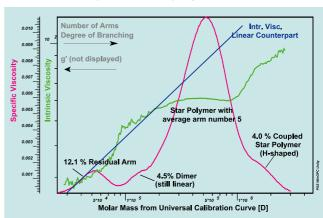
Validated and proprietary viscometry data processing methods derive true molecular weights and reliable Mark-Houwink constants based on the universal calibration principle. The branching index g' can be measured across the molar mass distribution.
