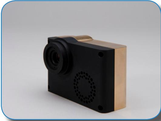
PPD detectors are compact and include all electronics required to detect single photons with picosecond accuracy. The module contains a wide bandwidth GHz pre-amplifier, picosecond timing constant fraction discriminator and regulated high voltage supply all in one compact, fully integrated package.
