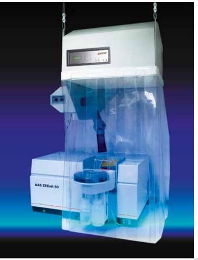
The instruments of the EFBS-V-series are being installed where clean room conditions are required but vapor, combustion gases, etc. may interfere. For example Graphite Furnace AAS, ICP, ICP/ MS, and most work areas in the chemical-analytical laboratory.
