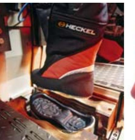
Attaching the sole to the shaft.
