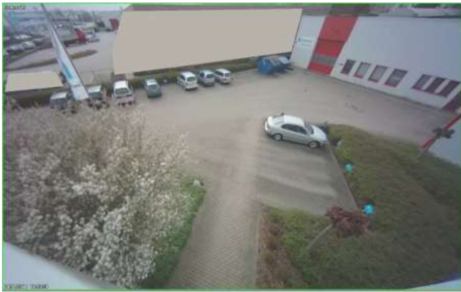
EQH 5200 with EFV 167 MP-DC, horizontal viewing angle ~ 116° (resolution 1280 x 720)
