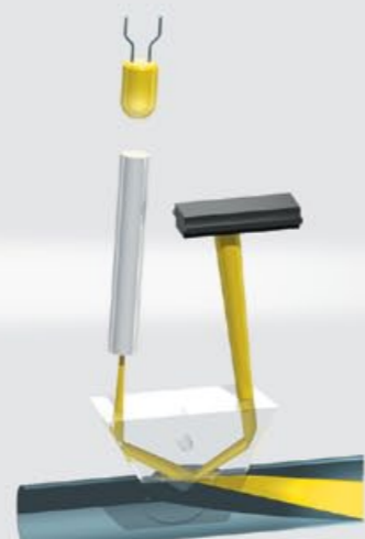
Demonstration of the function of a Process Refractometer
