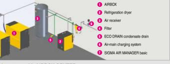
Compressed air system with AIRBOX CENTER
