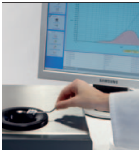
Simple feeding of the sample into the ultrasonic bath of the wet dispersion unit
