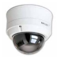
Basler IP Fixed Dome Cameras are especially energy efficient. All camera functions, including the fan and heater, can be powered using standard PoE (Power over Ethernet IEEE 802.3af Class 0). Basler IP Fixed Dome Cameras have a built-in micro SDHC card slot that can be used for local file storage.
