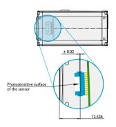
The back focal length on each camera is carefully measured and adjusted by our unique "CSAT" procedure. This guarantees an optimum distance between the lens flange and the sensor and ensures outstanding image quality based on compliance with optics standards.
