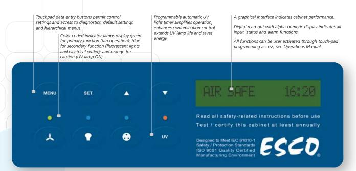
Sentinel Microprocessor Control System, Programmable When programmed ON • the start-up sequence confirms status with Air Safe and local time display. • the Personal Identification Number (PIN) access restricts unauthorized adjustments. • an airflow alarm warns of deviations from normal velocities.
