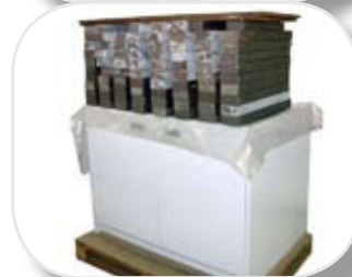
Cabinet Load Test
