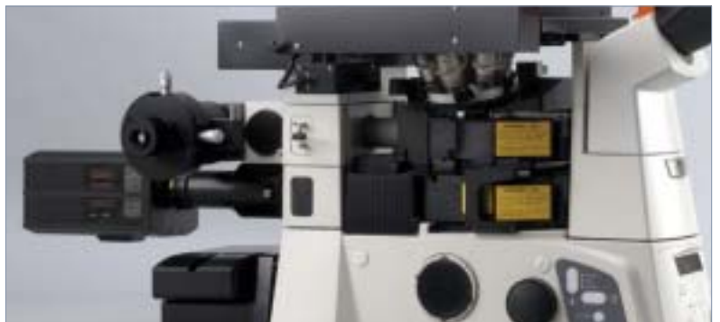
Example: In addition to the PFS, a photo activation module (upper tier) and a back port (lower tier) are mounted.
