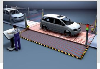
Guarding danger zones in expansive machinery systems for complete safety – even at points that are not visible.
