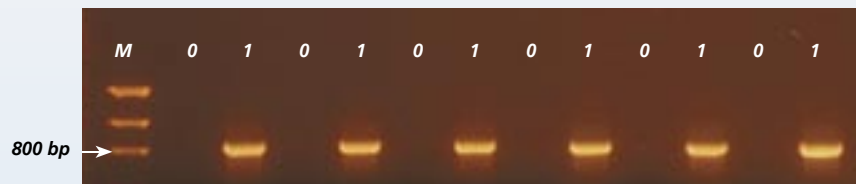
Figure 2: Evidence of cross-contamination-free pipetting. A NADH-dehydrogenase gene fragment from genomic wheat DNA was amplified via PCR. Low DNA Mass Ladder (M), PCR product without DNA (0) and with DNA (1) were separated on an agarose gel by electrophoresis.
