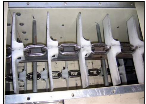
Bolt 'N' Go System Drop Forged Chain Application on a Conveyor
