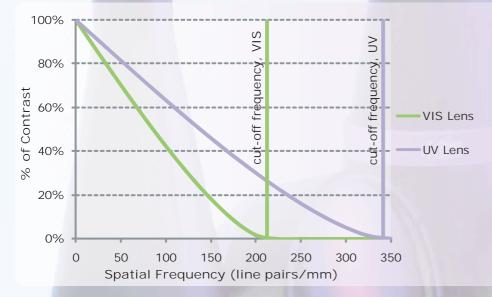
The graph on the left shows the limiting performances (diffraction limit) of two lenses operating at working Fnumber 8.
