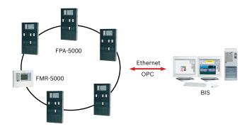
The FMR-5000 Remote Keypad offers the decentralized operation of a control panel or control panel network.
