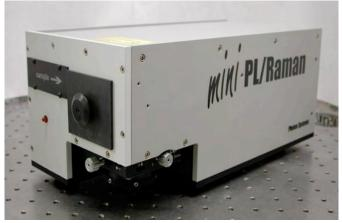
Measurement of photoluminescence (PL) spectra from semiconductor materials is an important characterization method and is widely accepted for providing information on carrier doping levels, alloy composition, bandgap and edge effects, etc. These measurements are important both for research, device characterization and process monitoring.
