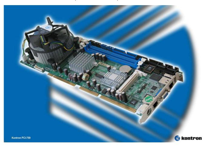
**Eching/Nuremberg, Germany, February 26, 2008** – Today, at Embedded Word (Hall 12 / Booth 404), Kontron introduced the new Kontron PCI-759 PICMG 1.0 slot-CPU board with Intel multi-core performance. The long time available Kontron PCI-759 offers outstanding processor performance at an excellent price/performance ratio for industrial grade embedded applications such as process control, test & measurement and vision systems.
