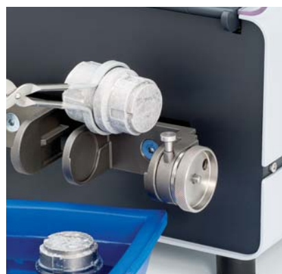
Before grinding, the jars are immersed in liquid nitrogen (-196 °C) in the cryo box for approx. 2 - 3 minutes
