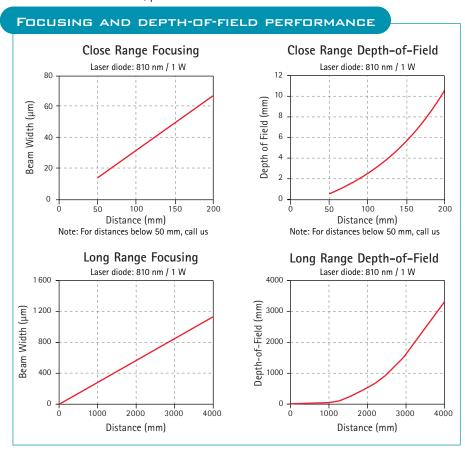
These charts are useful for establishing the smallest achievable line thickness and depth-of-field for your application.
