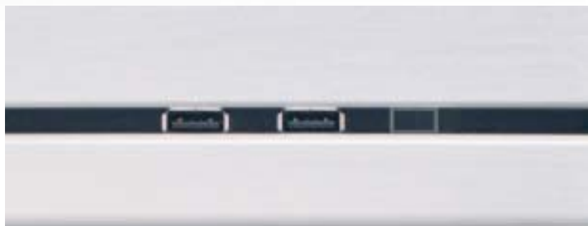
Directly on the front panel and therefore easy to reach: Simple connection of external discs with USB sockets. Quick triggering (eg off a backup) with extra switch.
