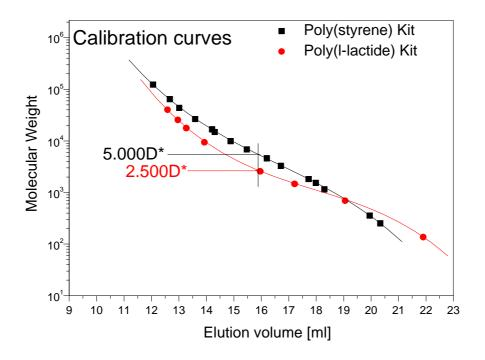
Comparison of a Poly(lactide) calibrated with Poly(styrene) black curve\* and with Poly(l-lactide) red curve\*. Up to 100% difference to the actual molar mass is possible
